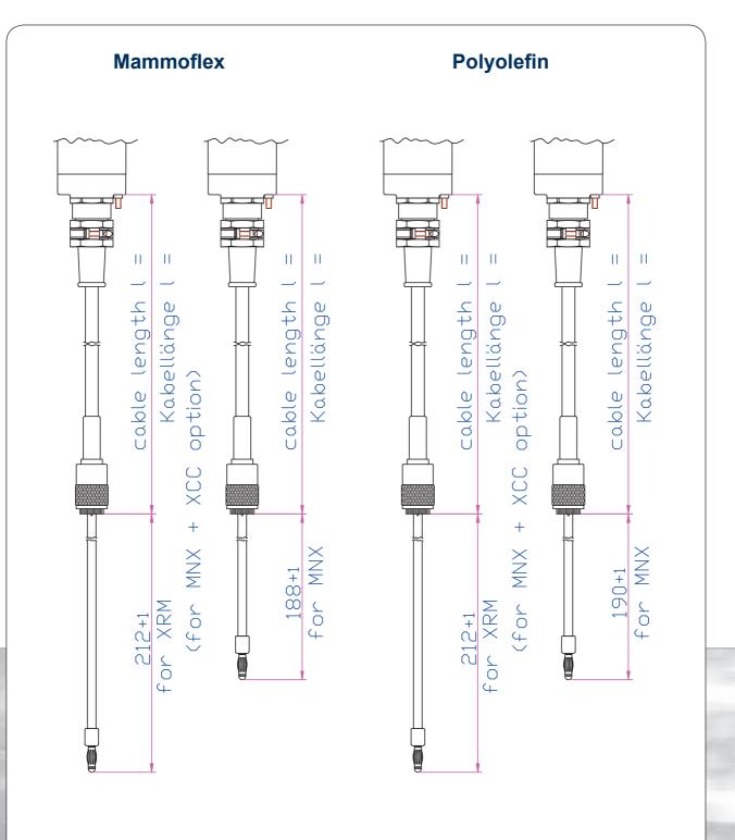
X-ray tubes of our MCB- and MCBM family are equipped with a glued in HT cable. The cable length as well as HT connector can be adapted according to the requirements of our customer and different power supplies.
